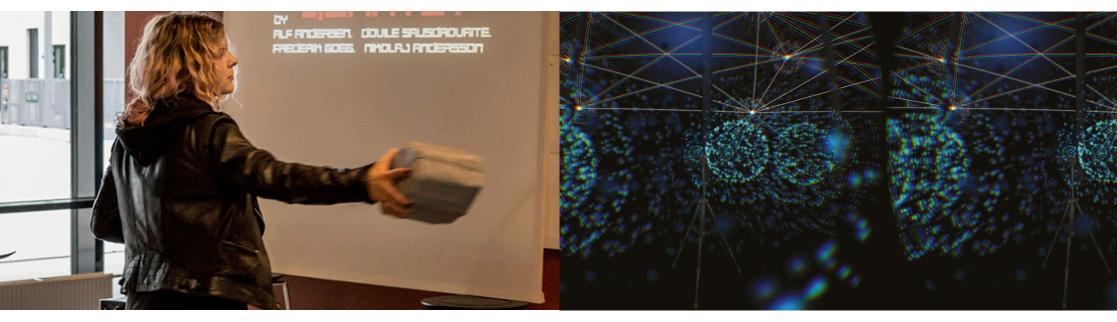
MONO Quartet is an installation of four gesture based digital instruments. The instruments produce noise music and sounds based on the movements of the performer. Each instrument sends sensory measurements wireless via bluetooth to a server arduino. The server sends MIDI through the serial port to a sound synthesizing computer.
